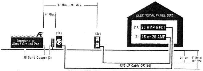
MUST BE THWN, XHHN, etc #12 WIRE IN CONDUIT (no UF cable) (1d)
