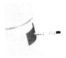
"NEC 2008 680.26(C) states: "An intentional bond of a minimum conductive surface area of 9" shall be installed in contact with the pool water. This bond shall be permitted to consist of parts that are required to be bonded in 680.26(B)."
